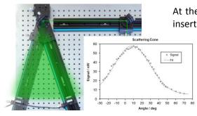
At the hinge angle connection a mirror or scattering discs can be inserted. The beam cone of reflected and scattered light is
