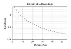
The necessary calculations for determination of the required safety distance for direct or scattered light of different laser sources is demonstrated and performed. Safety distances for the human eye and skin are calculated.
