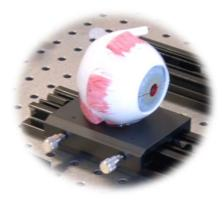
A model of an eye is inserted in a laser beam. Focusing of a laser beam by the lens onto the retina is performed. Thermal damaging of the retina is impressively demonstrated using an IR laser.
